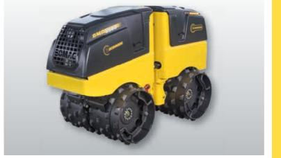
Areas of application: Soil compaction. Trench and pipeline construction, backfilling and foundation work - wherever high demands are placed on mobility, manoeuvrability and ease of operation coupled with difficult ground
