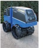
Displays degree of compaction in real time. Saves time and costs by avoiding unnecessary passes and always achieving optimum compaction. Warns of over-compaction and grain breakage and identifies weak points in the soil. BPR >350 kg, BMP 8500.
