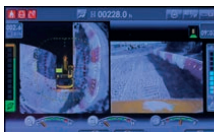
With KomVision, various camera view options are available whilst maintaining constant "birdview" from above the machine
