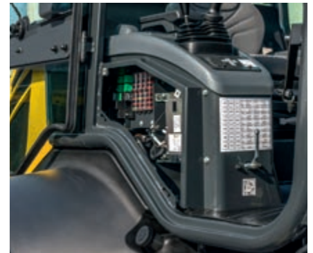
Side cover for quick maintenance access
