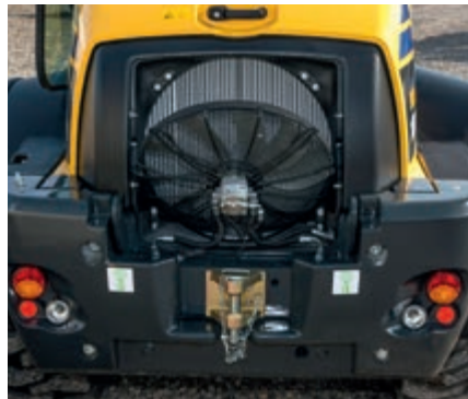
Tiltable radiator fan for convenient cleaning access
