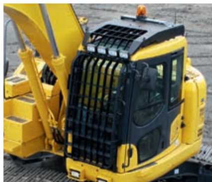
Falling Object Protection System (FOPS) optional
