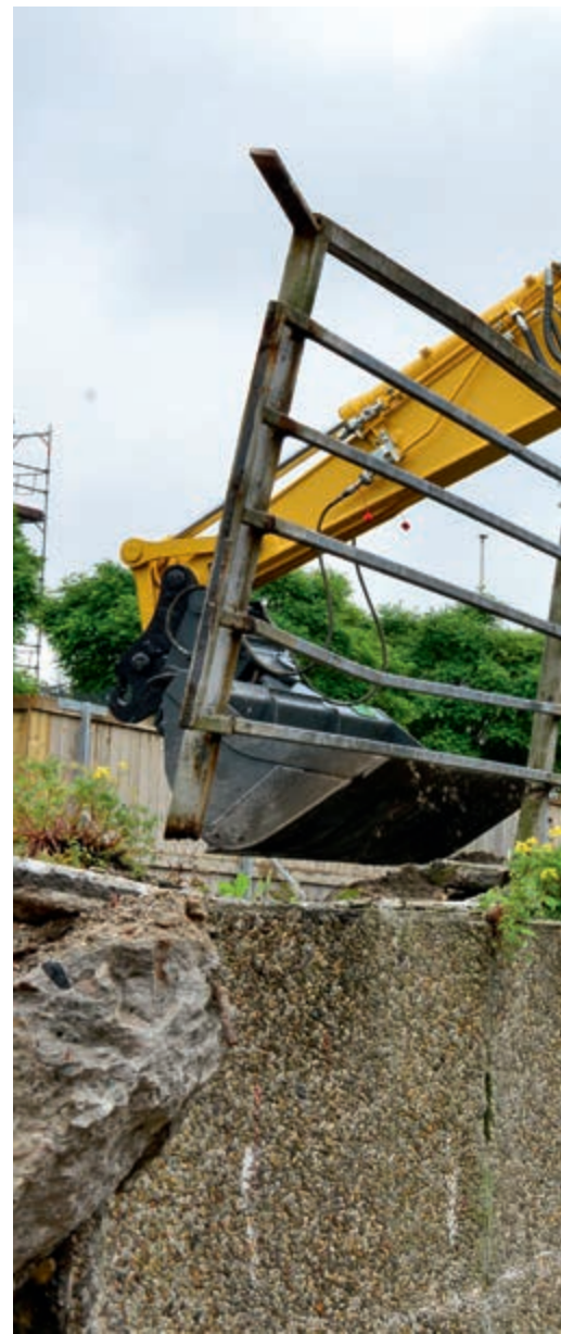
Falling Object Protection System (FOPS) optional
