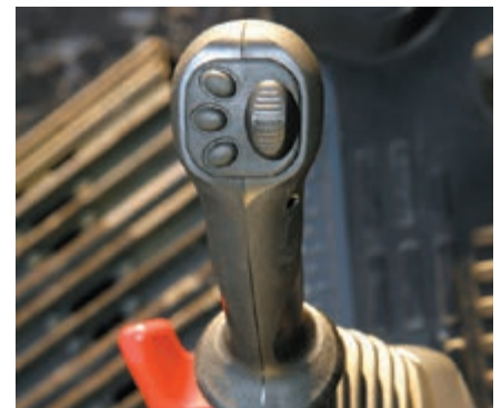
Joysticks with proportional control button for attachments
